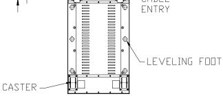
Figure 10 – "A" Battery Cabinet Drawing for 24/36kVA Ratings
